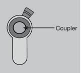
2. Turn the key until the cam is at 6 o'clock. Insert the profile half cylinder into the lock.
