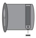
4. Drill a hole with a depth of 140-145 mm and a diameter of 50-55 mm in the wall or floor
